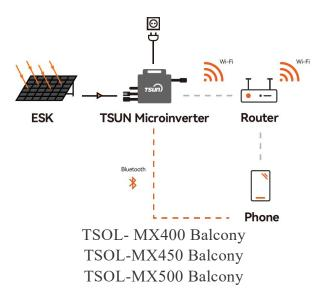
The microinverter is integrated with the Wi-Fi module and connects to the home Wi-Fi router directly. Users can monitor the power generation of the system by TSUN monitoring App.
